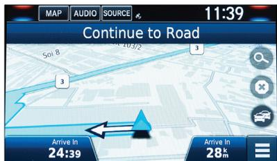
Step 7 – The system will calculate and display the route line on the map screen.
